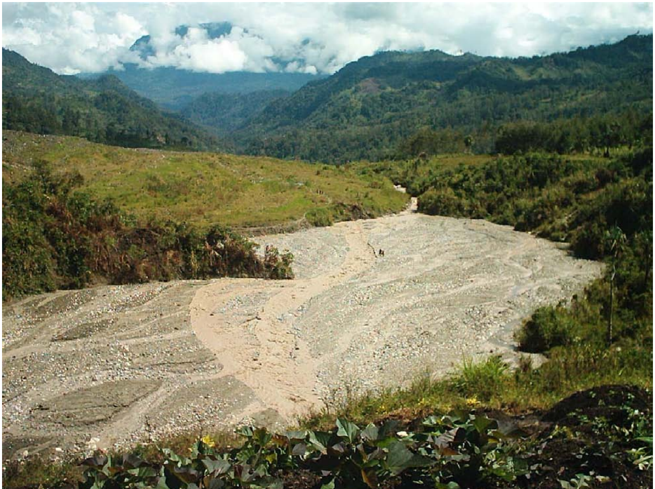
Tailing discharge at South Anawe erodible dumpsite.
